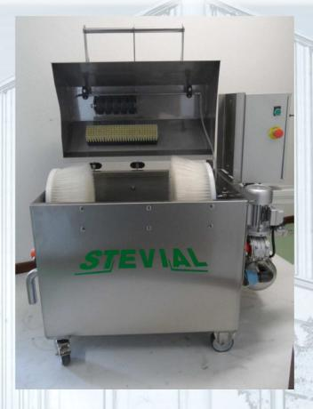
The washer has been made for the cleaning, by external brushing, of 20 to 50-liter beer barrels, without any adjustment. The cleaning rate depends on the time of the cycle that has been chosen.
